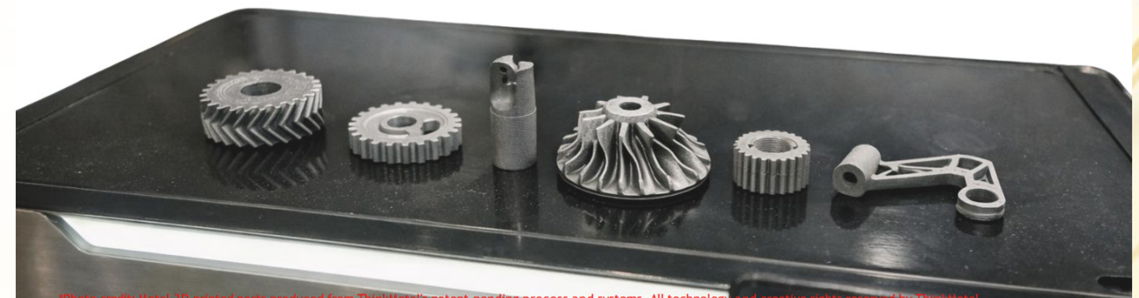
*Photo credit: Metal 3D printed parts produced from ThinkMetal's patent-pending process and systems. All technology and creative rights reserved by ThinkMetal.
