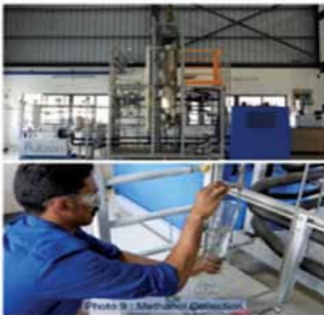
M/s Breathe Applied Sciences Private Limited, Bengaluru CO 2 conversion to methanol to the pilot scale
